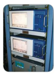
Toxic hydrocarbons can enter the atmosphere as part of the emissions of industrial enterprises for the production of polymers, drugs, oil refining, etc. This analyzer is designed to measure the content of hydrocarbons that have toxic and / or carcinogenic properties, as well as those involved in the formation of ozone.
